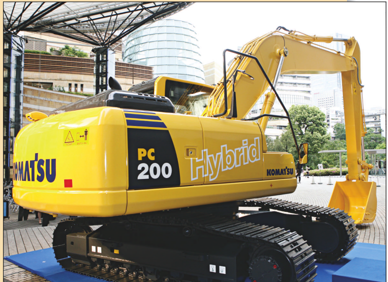
Capacitors store slewing energy to assist diesel power, cutting fuel consumption 25 percent.
